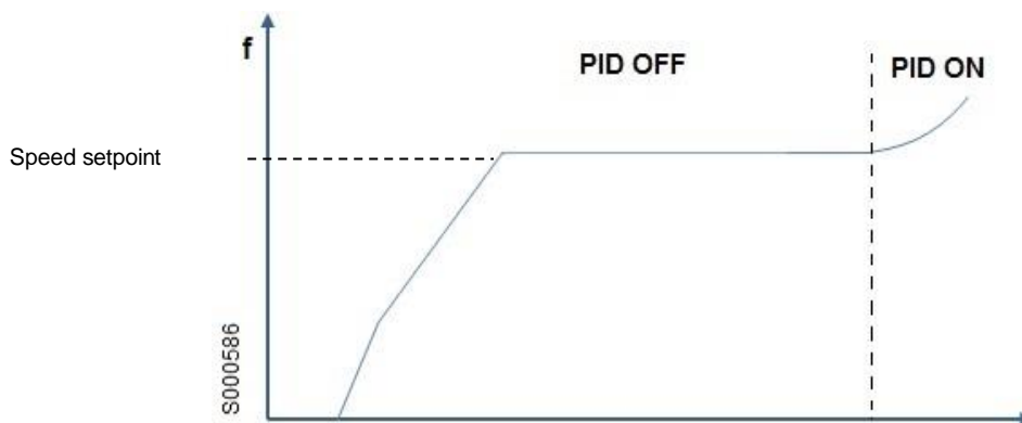
Figure 40: Ramp example – filling horizontal pipes
